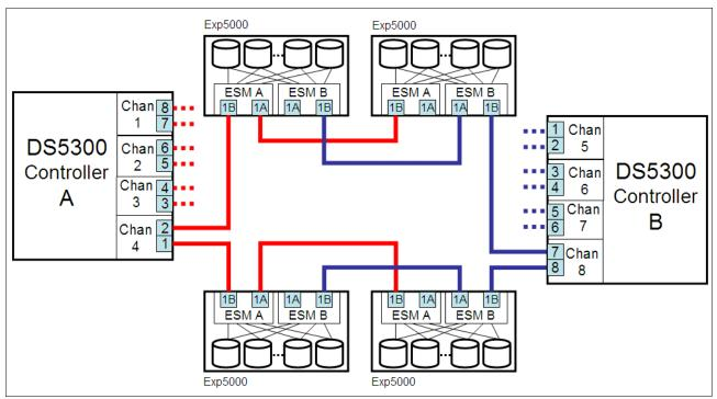
Figure 5-73 Drive-side connections
