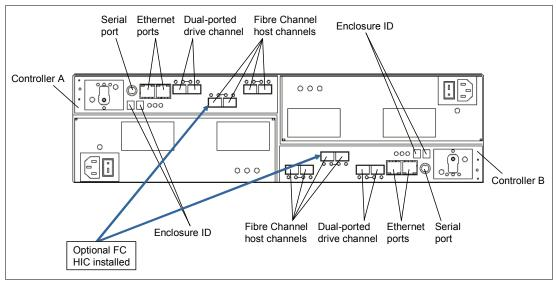
Figure 2-45 DS5020 rear view: 8 FC Port model
