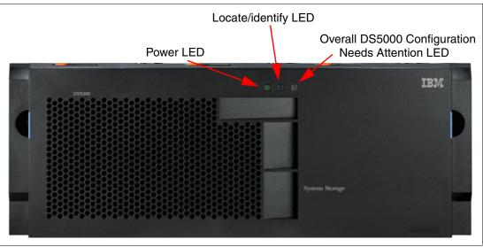
Figure 2-17 Front bezel LEDs
