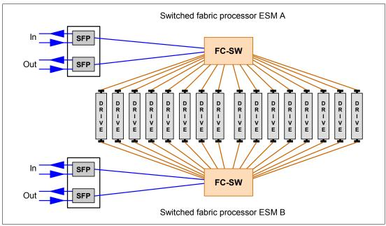
Figure 2-62 EXP5000 and EXP520 switched architecture
