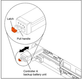
Figure 2-49 Replaceable Backup Battery Unit (BBU)
