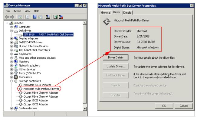
Figure 5-123 Determining the device driver in use
