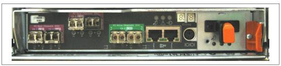
Figure 2-47 DS5020 controller photo rear view
