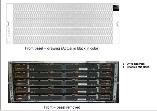
Figure 2-64 EXP5060 front bezel and drive drawers
