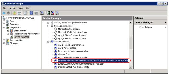
Figure 3-19 SM Failover (MPIO/DSM) Multi-Path Support
