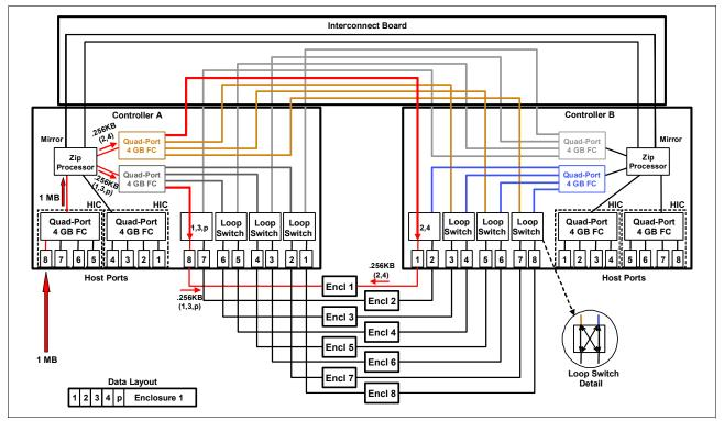
Figure 2-7 Data flow with one enclosure
