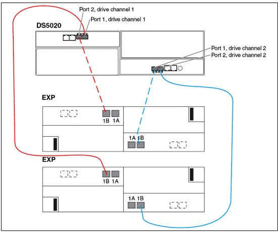
Figure 2-88 DS5020 drive cabling with two EXPs
