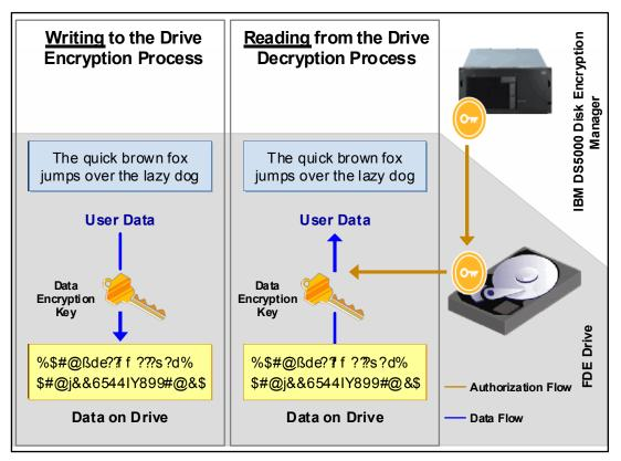
Figure 4-1 Full Disk Encryption using IBM Disk Encryption Manager and FDE drives
