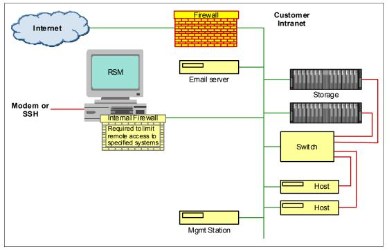
Figure 6-4 RSM internal firewall
