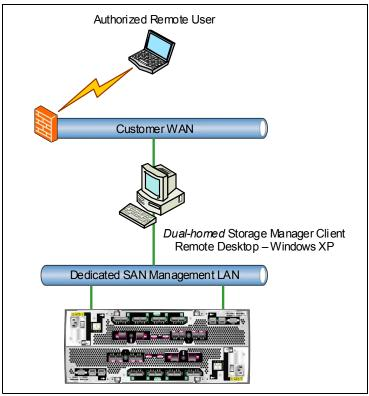
Figure 5-57 Securing remote access to the Storage Manager Client
