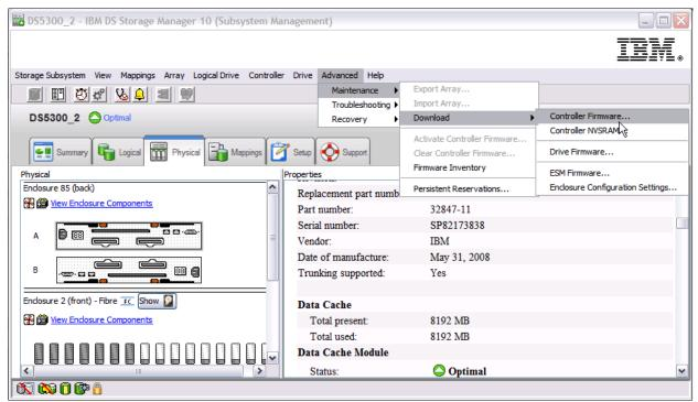
Figure 5-5 Subsystem Management window: Controller Firmware upgrade
