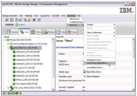
Figure 5-86 Check array redundancy
