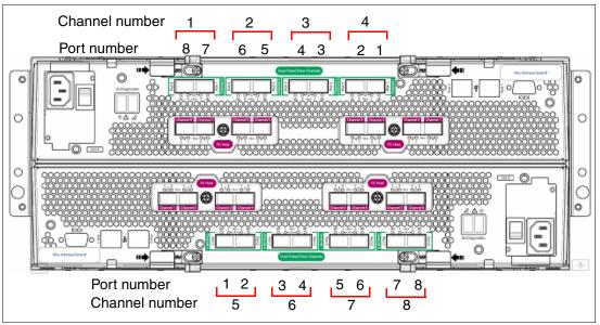
Figure 2-30 Disk drive channel and port numbering
