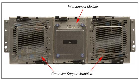
Figure 2-11 Front view of the DS5000 storage subsystem
