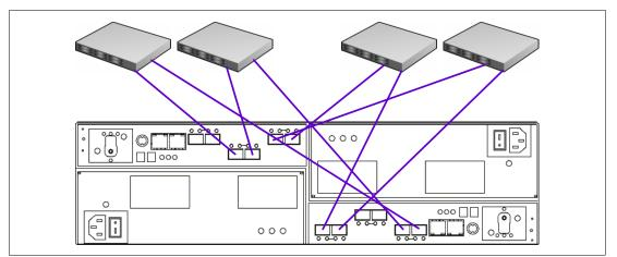
Figure 2-55 DS5020 mixed host connection layout
