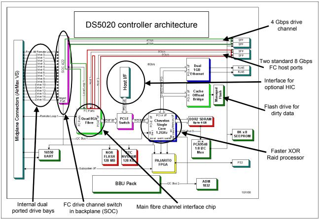
Figure 2-34 DS5020 controller architecture breakdown
