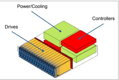
Figure 2-37 DS5020 hardware components
