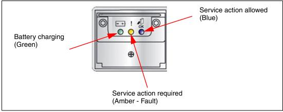
Figure 2-53 Battery LEDs
