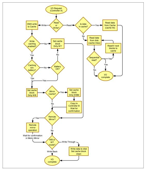
Figure 2-9 Simplified data cache flow diagram
