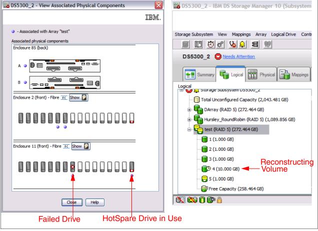
Figure 5-104 Storage Manager view after disk failure
