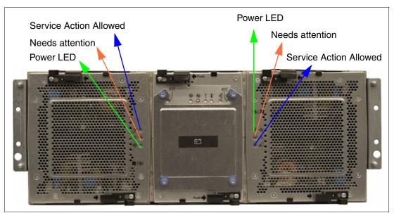
Figure 2-24 Controller support module (power supply/fan) LEDs
