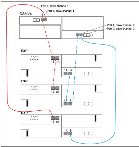
Figure 2-89 DS5020 drive cabling with three EXPs
