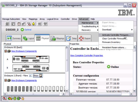
Figure 5-12 Activate staged firmware manually
