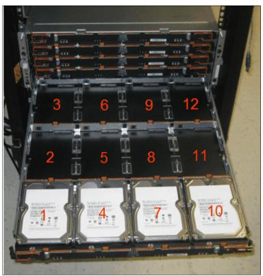
Figure 2-65 EXP5060 drawer with required drives shown
