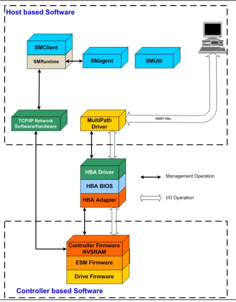
Figure 3-1 Storage Manager software components
