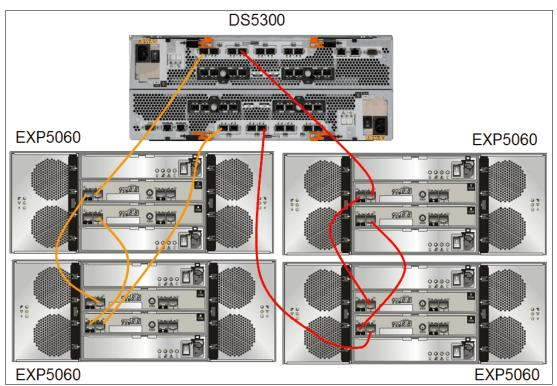
Figure 2-83 EXP5060 non-trunked and cascaded configuration
