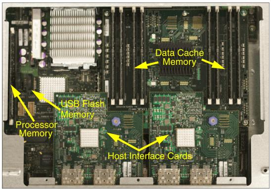
Figure 2-4 DS5000 controller with top lid removed
