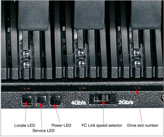
Figure 2-50 DS5020 front panel LEDs
