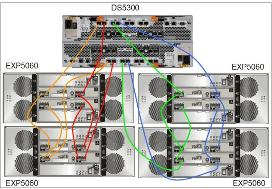
Figure 2-86 shows the four EXP5060s in a cascaded and trunked configuration.
