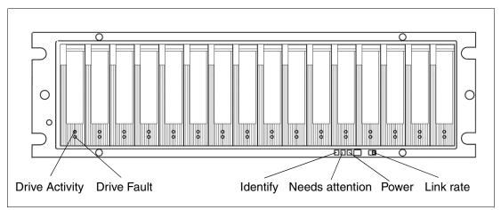
Figure 2-59 EXP5000 and EXP520 front panel
