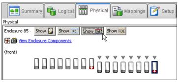
Figure 3-53 SATA drives protected with hot spare
