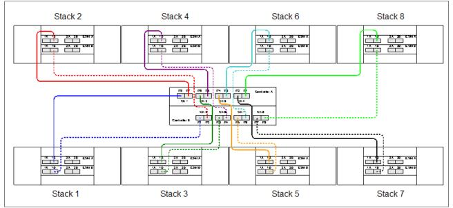
Figure 2-82 Cabling for non-trunked configuration of eight EXP5060s
