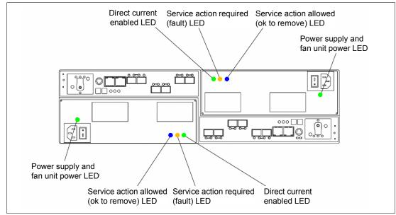
Figure 2-38 DS5020 power supply and fan unit LEDs
