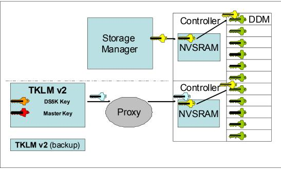
Figure 4-3 shows how keys are managed locally (top) or externally (bottom).
