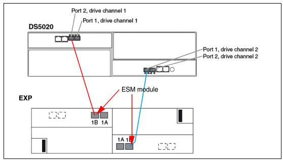
Figure 2-87 DS5020 drive cabling with one EXP
