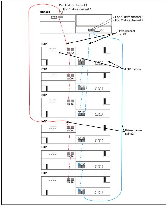
When six enclosures are required, the same method is employed again, maintaining drive channel redundancy and using both controllers, as shown in Figure 2-90.
