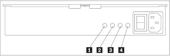
Figure 2-70 EXP5060 power supply LEDs
