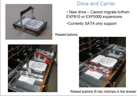
Figure 2-67 EXP5060 drive and carrier assembly
