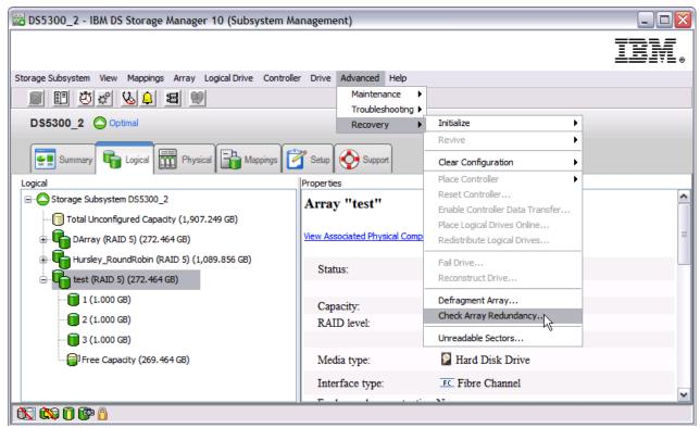
Figure 5-83 Check of array redundancy
