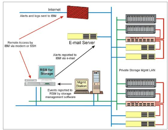
Figure 6-2 RSM for Storage connection
