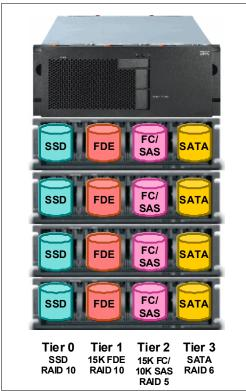
Figure 1-4 Multi-Tier HDD layout
