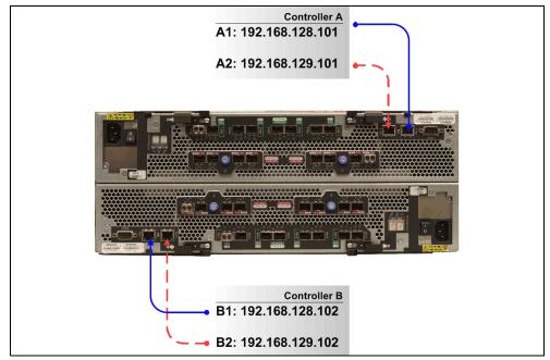
Figure 3-20 DS5000 storage subsystem default IP addresses
