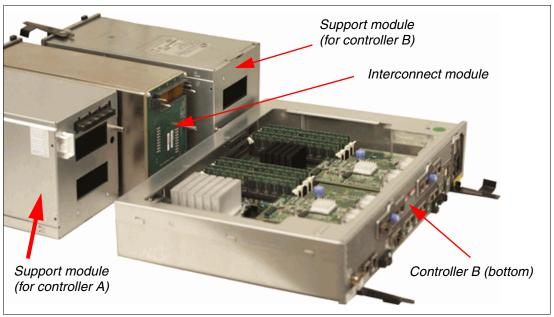
Figure 2-13 shows a DS5000 storage subsystem without a chassis (controller A is removed).
