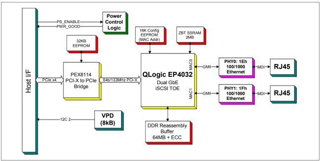
Figure 2-36 DS5020 iSCSI HIC architecture
