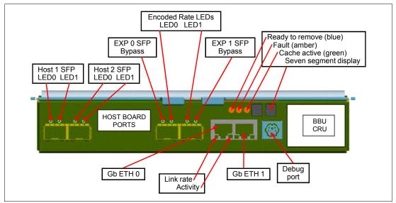
Figure 2-51 DS5020 RAID controller LEDs
