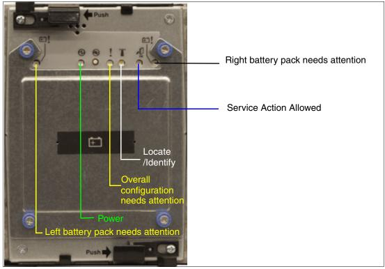
Figure 2-25 Interconnect module LEDs
