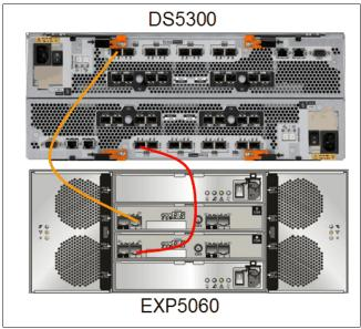
Figure 2-81 EXP5060 cabled non-trunked to the DS5300
