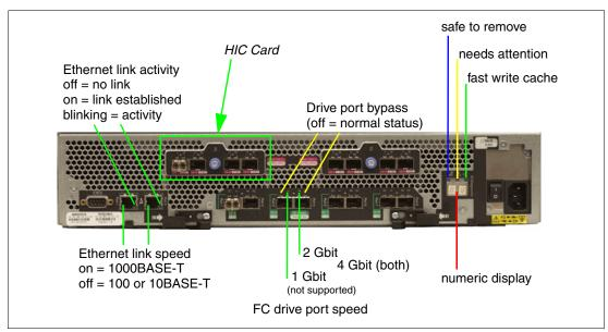
Figure 2-18 RAID controller LEDs (controller B): FC HIC version
