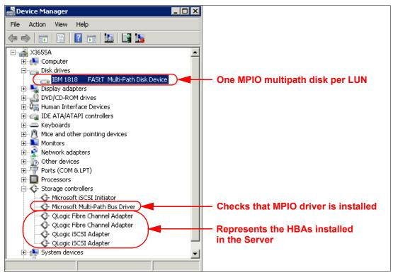
Figure 5-125 Device representation either using MPIO or SDDDSM
