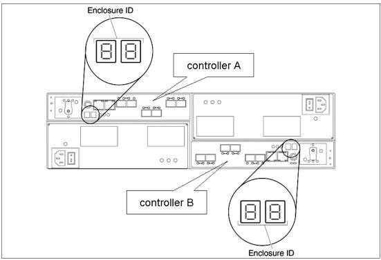
Figure 2-52 DS5020 controller enclosure ID display
