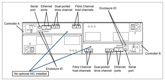
Figure 2-44 DS5020 rear view: Base model
