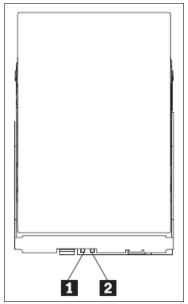
Figure 2-68 EXP5060 DDM LEDs
