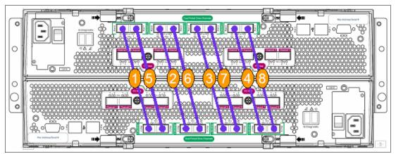
Figure 2-31 Enclosure connections order
