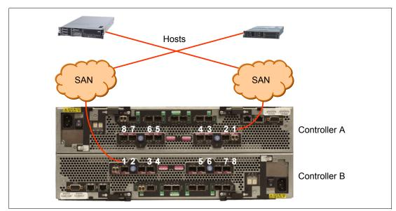
Figure 2-27 SAN connected hosts to DS5000 storage subsystem
