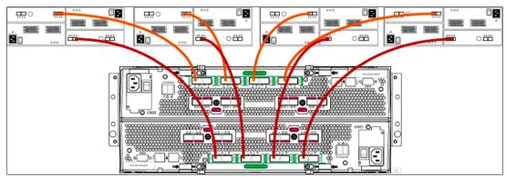
Figure 2-74 DS5000 with four expansion units
