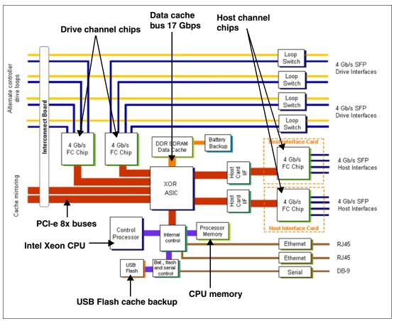
Figure 2-3 shows the main components of the DS5000 controller.
